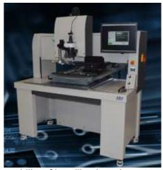
Also highlighted will be the Summit LXi/LT120 systems with capability of handling boards up to 650 x 1200 mm and components up to 120 mm.
