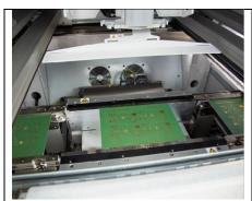
Three-stage conveyor system: While one board is being printed, the previously printed board is moved out of the machine and the next board moved into the machine.
