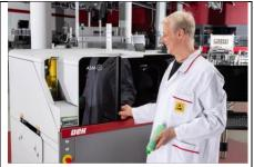
Fewer line stops: The optional Dual Access Cover makes it possible to replace paste cartridges without having to stop the printer.
