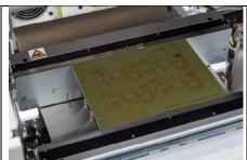
DEK All-Purpose Clamping (APC): The by far most flexible DEK clamping system features jobspecific programming, saves time and effort, and offers significantly more capabilities.
