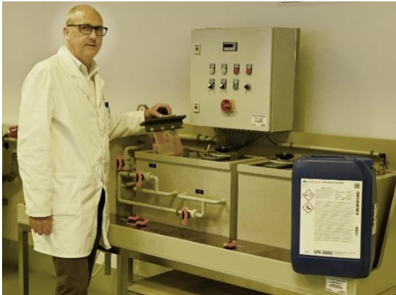
Johannes Tekath in front of the new Peters-test unit handling a specimen holder. To the right, a can with the respective pre-treatment product supplied by Atotech.
