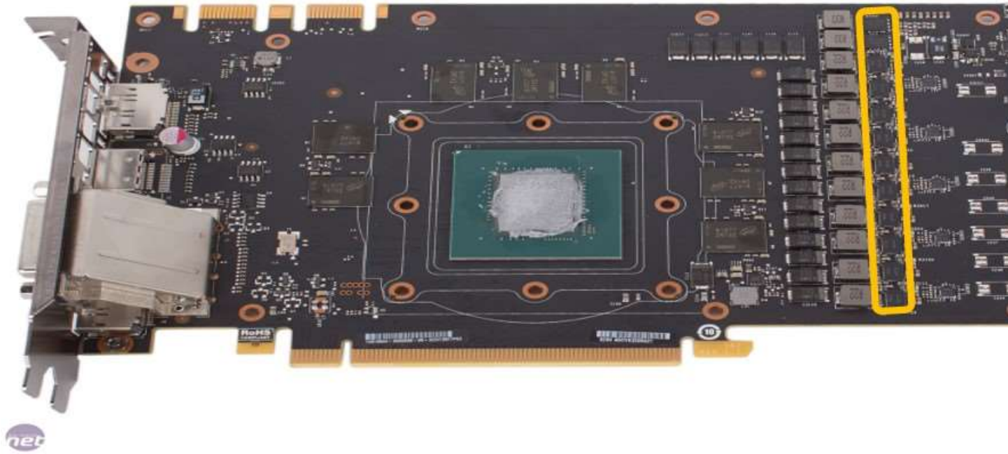
Figure 4b: GeForce-GTX-1080 EVGA card with 6 X 5 DrMOS MOSFETs (forums.evga.com)
