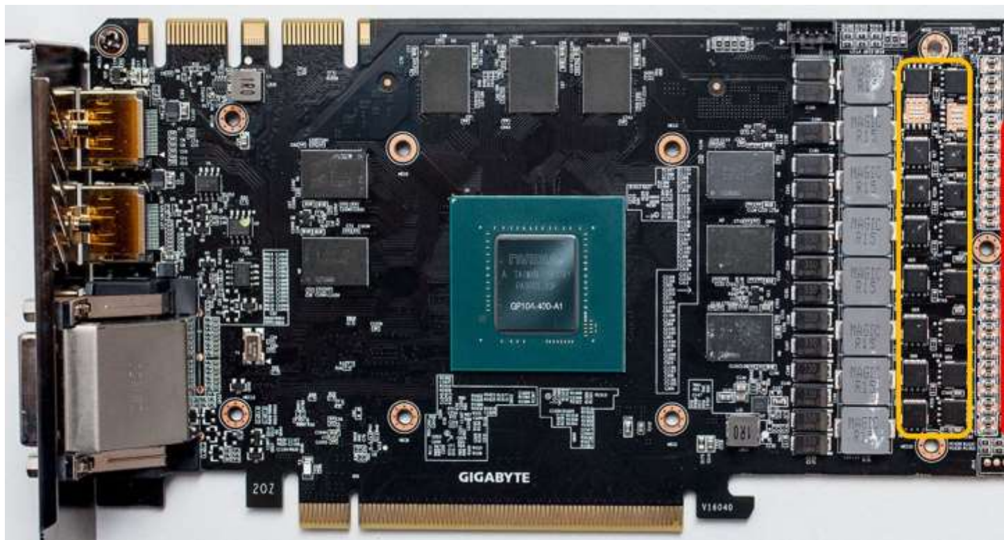
Figure 4a: GIGABYTE-GeForce-GTX-1080 VGA Card with Discrete MOSFET and driver IC
