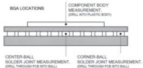
**Figure 3: TC location example for BGAs.**
