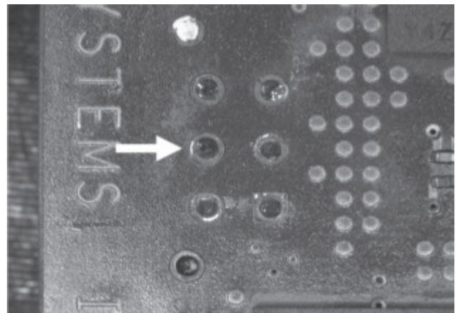
Figure 6: Cu dissolution of PTH barrels using SAC alloy
