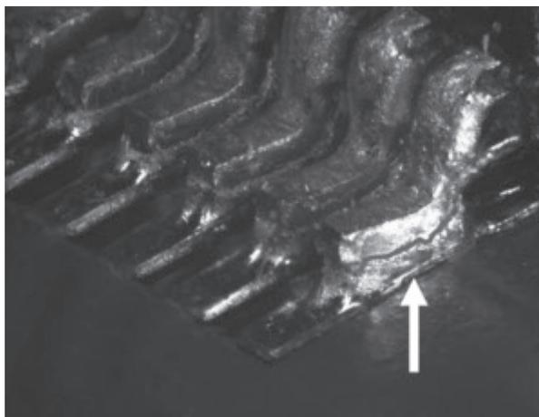
**Figure 8: TSOP solder joint thermal fatigue failure**
