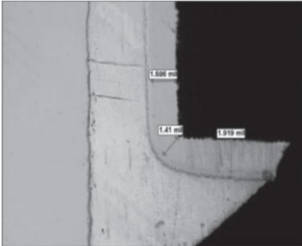
**Figure 7: Alternate alloy solder fountain cross section**
