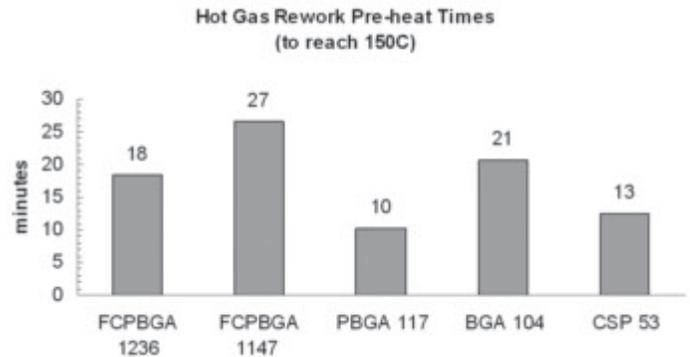
Figure 5: Long pre-heat times for lead-free BGA rework
