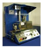
Finally we will consider methods and equipment available for applying conformal coatings. There are many suppliers of dipping equipment used to apply conformal coatings - a wide range of sophistication and prices is available. It is important with dipping to carefully control withdrawal speed as this will determine coating thickness - the slower the withdrawal speed, the thinner will be the resultant coating. Coating thickness will also be determined by other factors such
